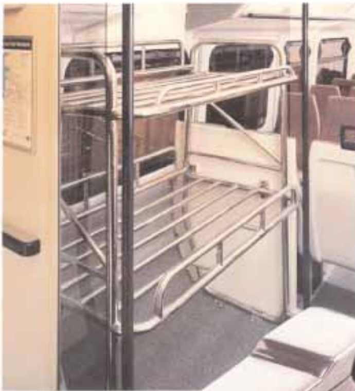
Above: Stainless luggage rack fitted to a class 323 DMU for Manchester Airport.
