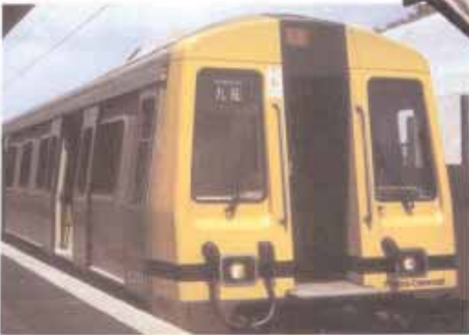
Below: Stainless steel cab door handrails fitted to a Kowloon Locomotive.
