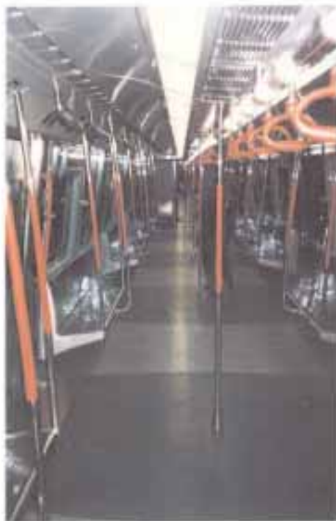
Above: Handrails supplied to the KCRC line Hong Kong. Stainless steel handrail poles with red nylon coated Abras tube grips.
