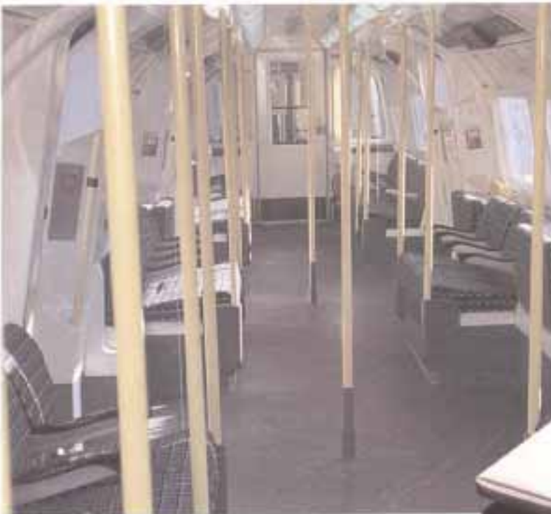
Above: Nylon coated handrail poles and fittings to the London Underground Northern Line rolling stock.
